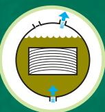
3 Hydraulic pressure applied, forcing the preservative deep into the structure of the timber.
