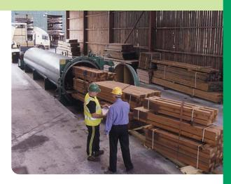
Tanalised® E pressure treated timber is timber which has been impregnated with Tanalith® E wood preservative under rigidly controlled conditions in a vacuum pressure timber impregnation plant.
